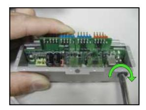
2. Position the I/O board into the bay with the component side to the left (close to the HDDs). Connect the I/O cables to the connectors on the back of the I/O board.
